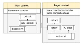
Figure 1: Having multiple build contexts is necessary to cross-compile OCaml projects.
